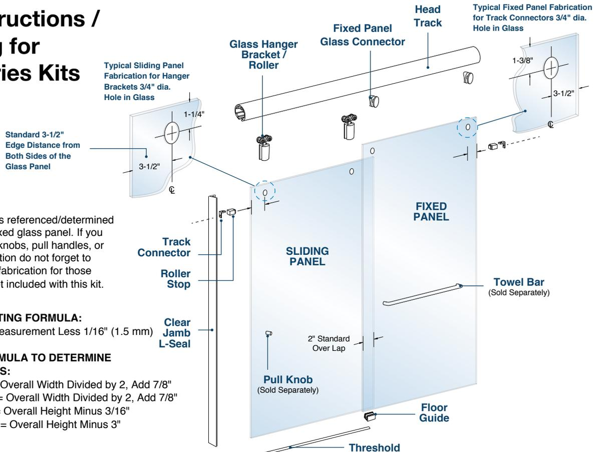
**NOTE:** The overall height is referenced/determined from top of curb to top of fixed glass panel. If you are including shower door knobs, pull handles, or a towel bar on your installation do not forget to allow for the required hole fabrication for those additional items that are not included with this kit.
